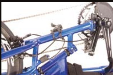
Fork is super stiff with an ovalized upper tube, longer headtube, 2" of vertical adjustment and a bicycle headset. Plus its easier than ever to remove the fork for travel
